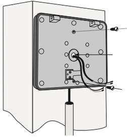
**Step 2:** Determine how the wires will enter the keypad (e.g., from the back through a hole drilled in the post; running the wire on the post surface). Drill a hole in the back of the keypad cover and pull the wire into the cover. Then mount the cover to the post using the screws provided. Run wire through PVC pipe from the ground to keypad and from the ground to the opener control board to protect it from lawn mowers or grazing animals.
