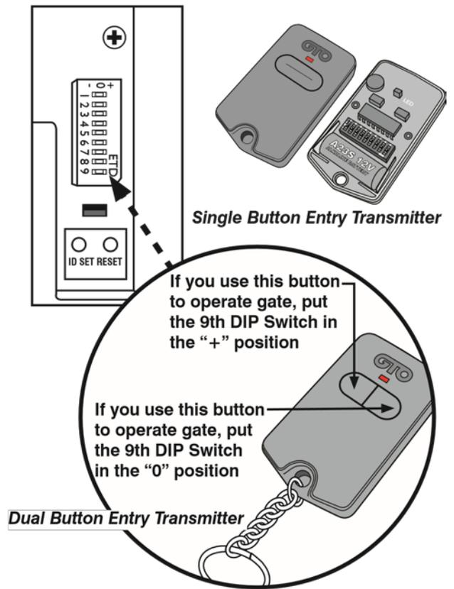
**Change the Keypad's DIP Switch Settings NOT the Entry Transmitter Dip Switch Settings**
