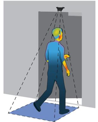
Reduces False Detections by Detecting Both Presence and a Change in Temperature
