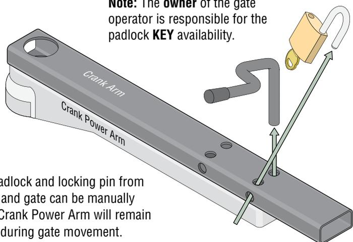
Remove padlock and locking pin from crank arm and gate can be manually operated. Crank Power Arm will remain stationary during gate movement.
