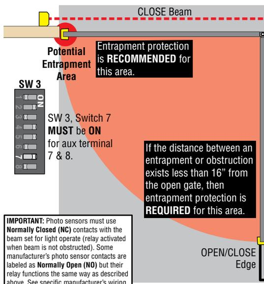
**IMPORTANT:** Photo sensors must use **Normally Closed (NC)** contacts with the beam set for light operate (relay activated when beam is not obstructed). Some manufacturer's photo sensor contacts are labeled as **Normally Open (NO)** but their relay functions the same way as described above. See specific manufacturer's wiring manual for more information about their specific relay function.
