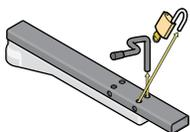
**2. In the event of a primary (AC) power failure and a back-up system (DC) power failure** (low charged or dead batteries for example), the system must have a release system to allow the gate to be **Manually Operated**.
