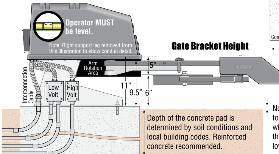
Depth of the concrete pad is determined by soil conditions and local building codes. Reinforced concrete recommended.
