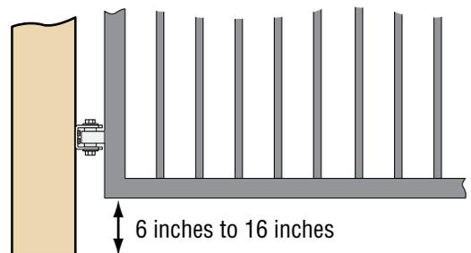
If bottom of gate is 6" to 16" above the ground at any part of the gate's traveling path, entrapment protection for this area is required.
