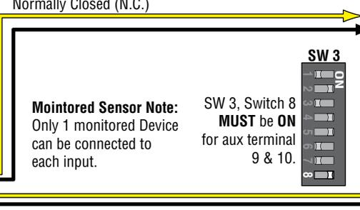
**Monitored Sensor Note:** Only 1 monitored Device can be connected to each input.
