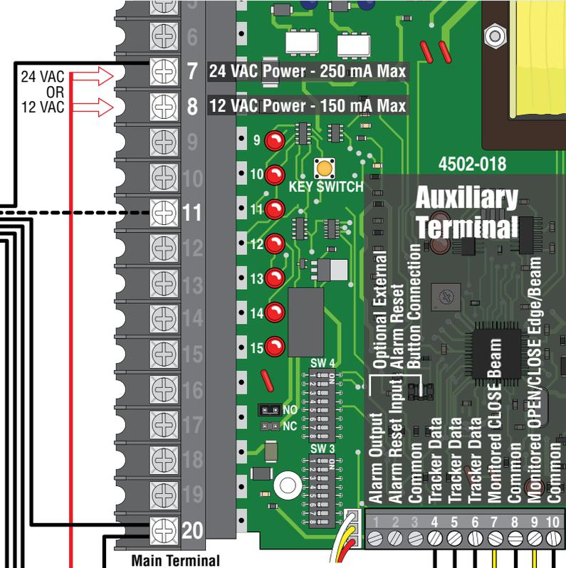
**External Entrapment Protection Devices:** In addition to the inherent reversing sensor system, this operator has a 10-pin Aux terminal for the connection of photo sensors-Type B1 and/or reversing edge-Type B2 entrapment protection required for UL 325 standards.
