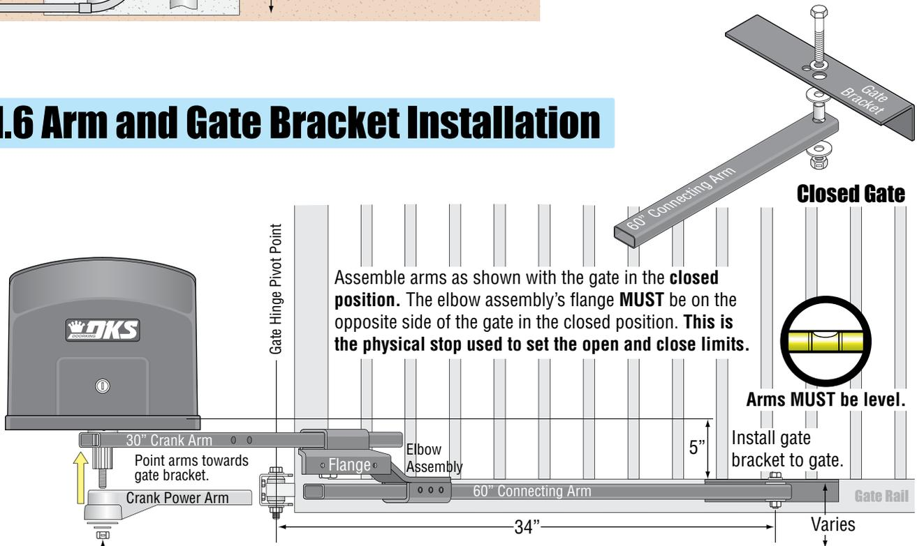
Assemble arms as shown with the gate in the **closed position**. The elbow assembly's flange **MUST** be on the opposite side of the gate in the closed position. **This is the physical stop used to set the open and close limits.**
