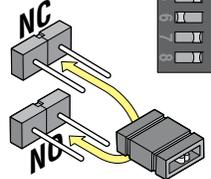
Contact rating is 1 amp maximum at 24-volts DC.
