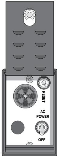
**To Manually Release Arm,** turn AC power to the operator OFF.
