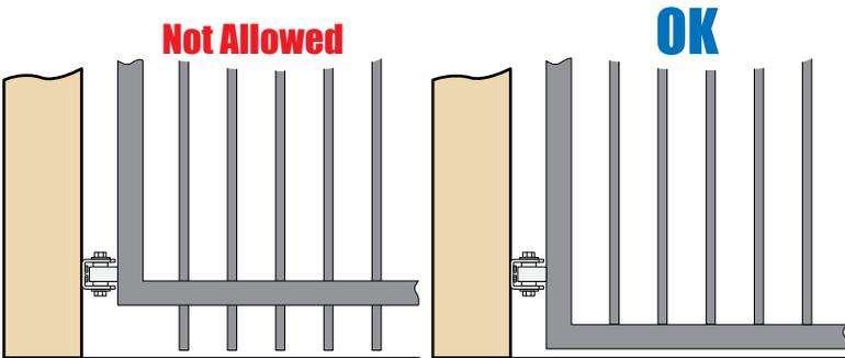
Gates shall have smooth bottom edges, with vertical bottom edged protrusions not exceeding 0.50 inches.
