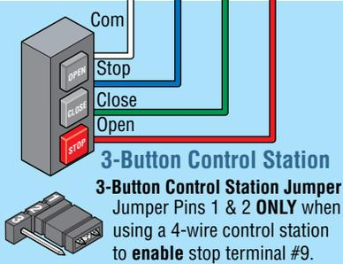
**3-Button Control Station Jumper Pins 1 & 2 ONLY** when using a 4-wire control station to **enable** stop terminal #9.
