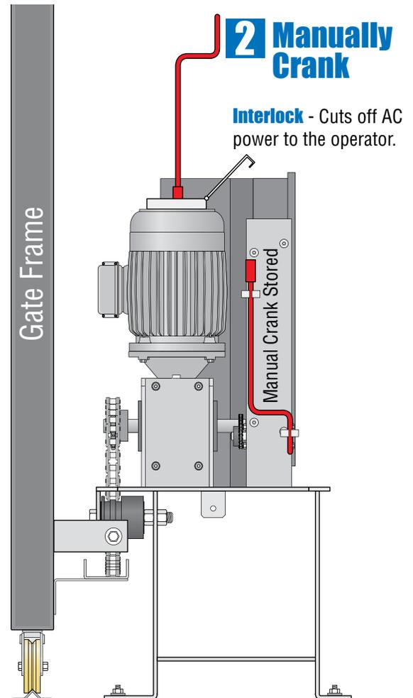
Insert the supplied manual hand crank into the motor shaft underneath the interlock door. Turn the crank to open the gate. Mechanical disc brake on 9555/9556 operator **MUST** also be manually released before manually turning the hand crank.
