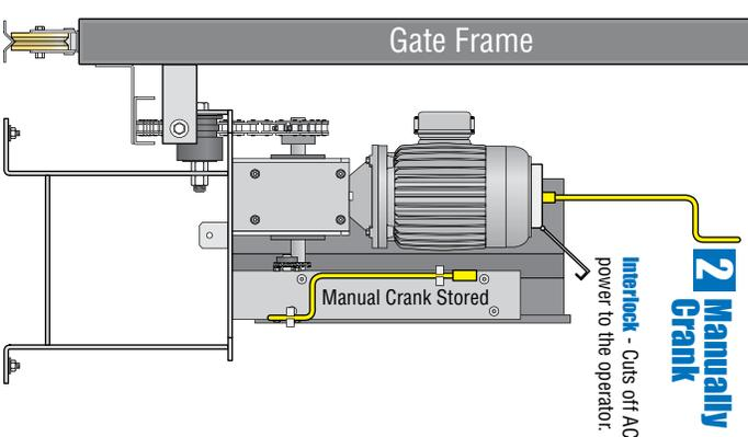
Insert the supplied manual hand crank into the motor shaft underneath the interlock door. Turn the crank to open the gate. Mechanical disc brake on 9555/9556 operator **MUST** also be **manually released** before manually turning the hand crank.
