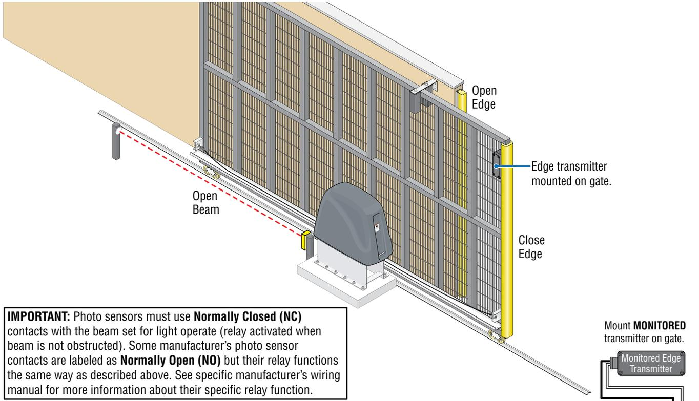
**IMPORTANT:** Photo sensors must use **Normally Closed (NC)** contacts with the beam set for light operate (relay activated when beam is not obstructed). Some manufacturer's photo sensor contacts are labeled as **Normally Open (NO)** but their relay functions the same way as described above. See specific manufacturer's wiring manual for more information about their specific relay function.
