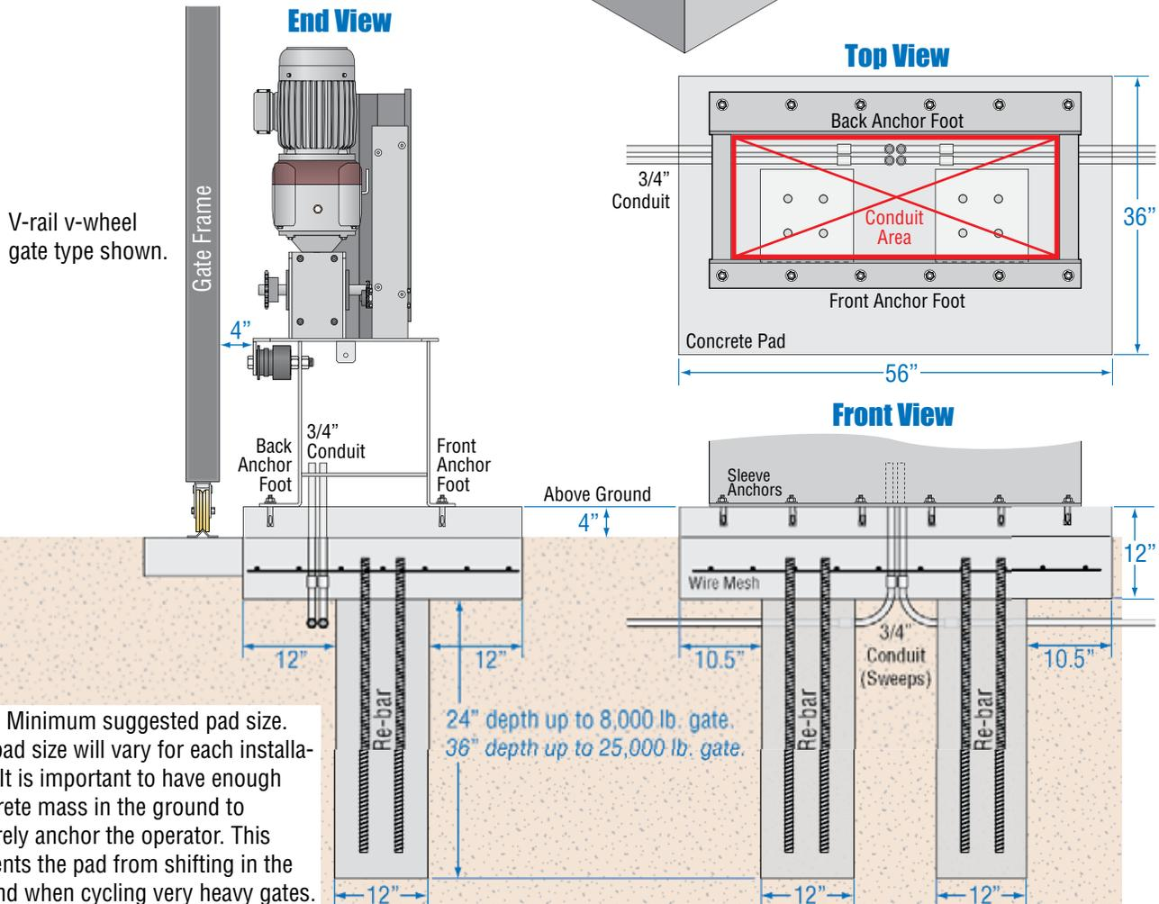
Note: Minimum suggested pad size. The pad size will vary for each installation. It is important to have enough concrete mass in the ground to securely anchor the operator. This prevents the pad from shifting in the ground when cycling very heavy gates.
