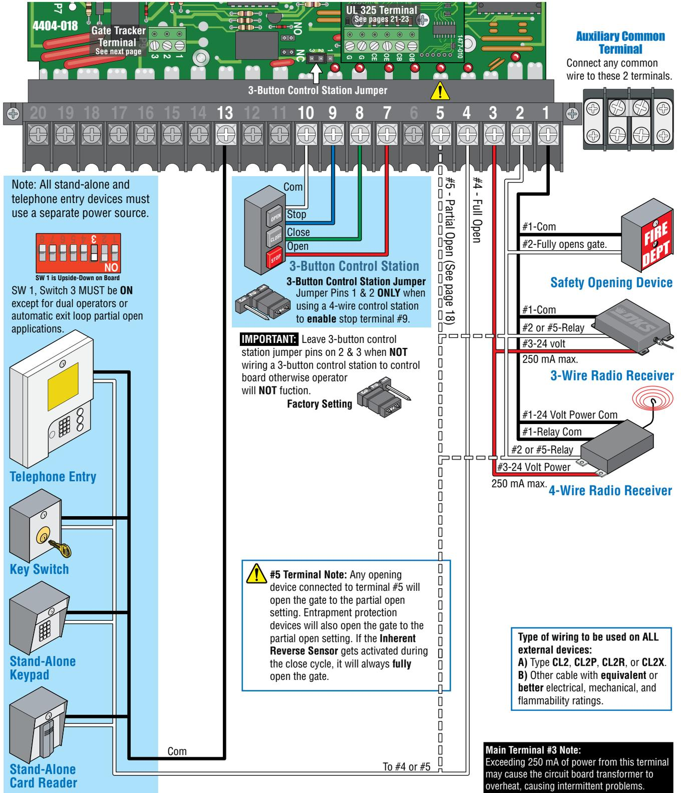
Note: All stand-alone and telephone entry devices must use a separate power source.
