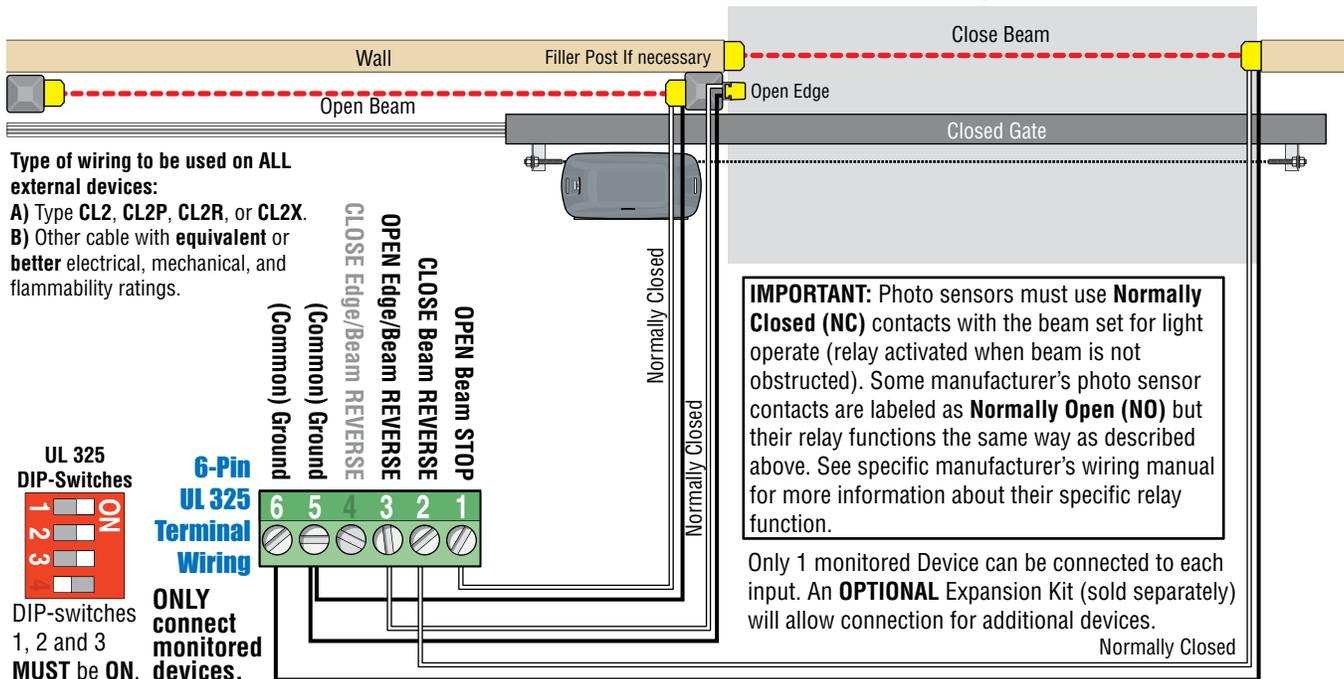
**Photo Sensor Power Note:** Photo sensors can be powered by the built-in convenience outlets located on the operator (See previous page).
