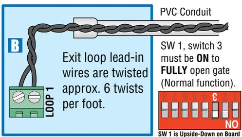
Note: The plug-in exit loop detector can be wired to partially open the gate if SW 1, switch 3 is turned OFF. A jumper wire must be connected from terminal #4 to terminal #5 (See next page for more information).
