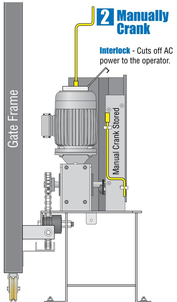
Insert the supplied manual hand crank into the motor shaft underneath the interlock door. Turn the crank to open the gate.
