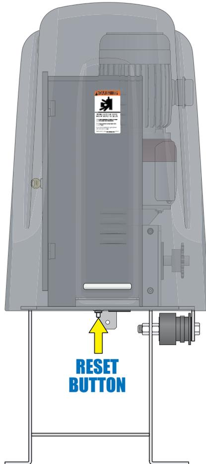
Press **RESET BUTTON**. This will reset the gate operator and allow normal gate operation again. **Accessible without removing the cover.**
