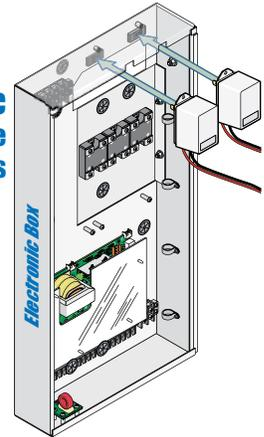
**Monitored Device Note:** Only 1 monitored Device can be connected to each input. An **OPTIONAL** Expansion Board (sold separately) will allow connection for additional devices.
