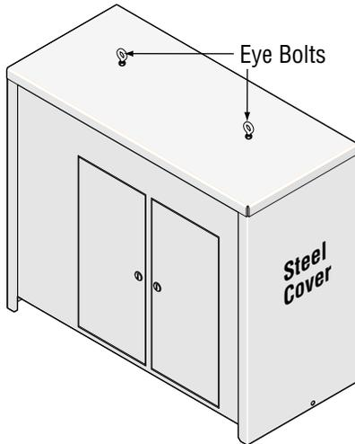
**OPTIONAL Steel Cover - DO NOT** lift gate operator using the eye bolts on top of cover or damage will occur. Only lift cover off operator.
