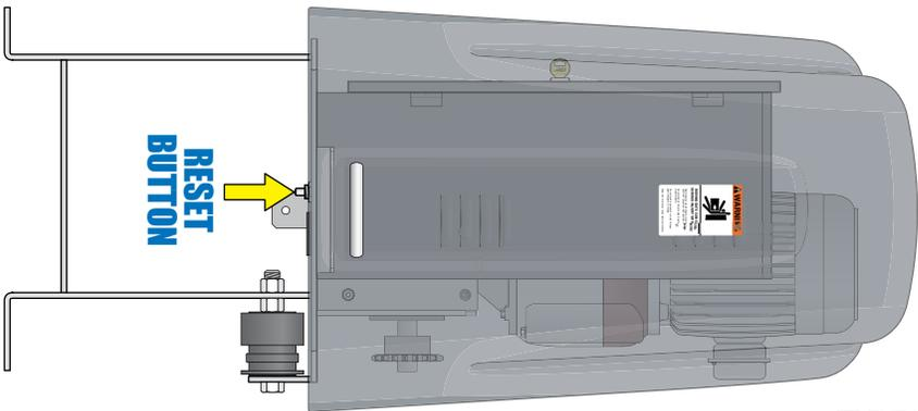
Press **RESET BUTTON**. This will reset the gate operator and allow normal gate operation again. **Accessible without removing the cover.**
