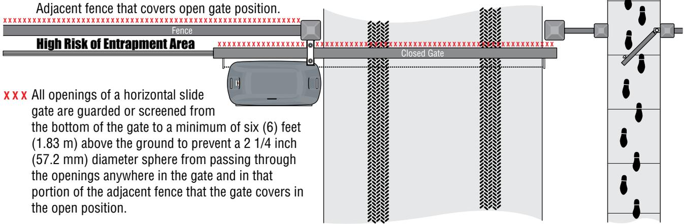
**XXX** All openings of a horizontal slide gate are guarded or screened from the bottom of the gate to a minimum of six (6) feet (1.83 m) above the ground to prevent a 2 1/4 inch (57.2 mm) diameter sphere from passing through the openings anywhere in the gate and in that portion of the adjacent fence that the gate covers in the open position.
