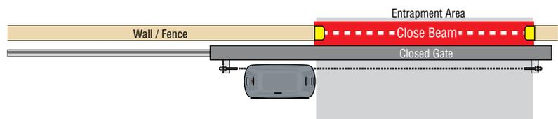
**3 OPEN Edge/Beam Reverse:** Obstructed reversing edge or photo beam will reverse the gate to the close position **during the opening-direction only**.
