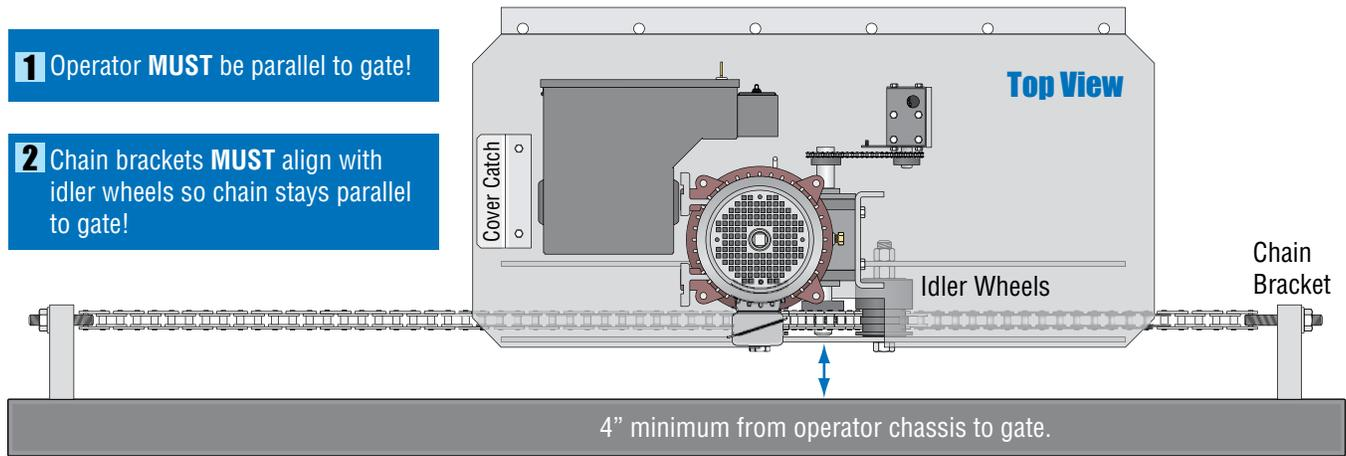
Note: Be sure to follow all 3 guidelines. Installing the chain in any other manner will cause excessive noise, chain idler wheel wear and chain stretching.
