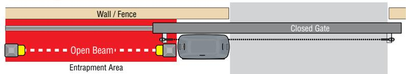
**2 CLOSE Beam Reverse:** Obstructed closing-direction photo beam will reverse the gate to the open position and reset the close-timer **during the closing-direction only**. Gate will close when timer times out.
