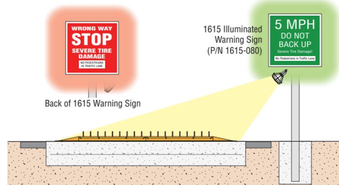
Additional lighting, warning signs and pavement markings can be used to increase awareness for potential danger and to separate pedestrians from vehicular traffic.
