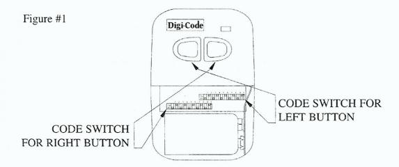
Once your have removed the battery hatch, locate the "CODE SWITCHES" above the battery. As shown above, the left button is controlled by the right hand switch and the right button is controlled by the left hand switch.
