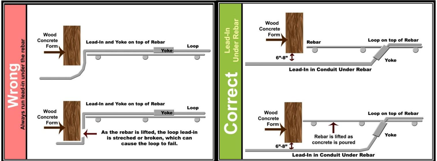
In the picture to the right notice how the "Correct" loop is offset from the rebar pattern. The loop is coming in contact with the rebar as little as possible. ----->
