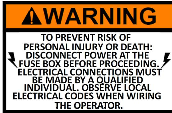
**WARNING:** These operators have been designed and constructed for use with voltages from 115 to 460 VAC. Check the operator nameplate label on the control box cover for the proper voltage and phase. The application of an improper input voltage or phase will result in catastrophic failure to the internal electrical components.
