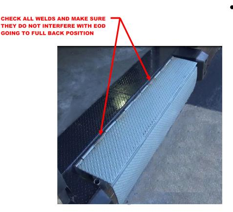
When the EOD is in the back position, verify that the welds at the tubes and the welds to weld the mounting plate to the dock do not interfere
