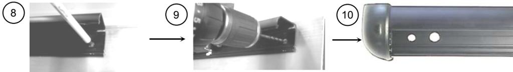
**NOTE:** Take care to avoid screw holes near the seams of the door, where it may be difficult to drill and install a screw, and possibly damage the inside structural braces of the door.
