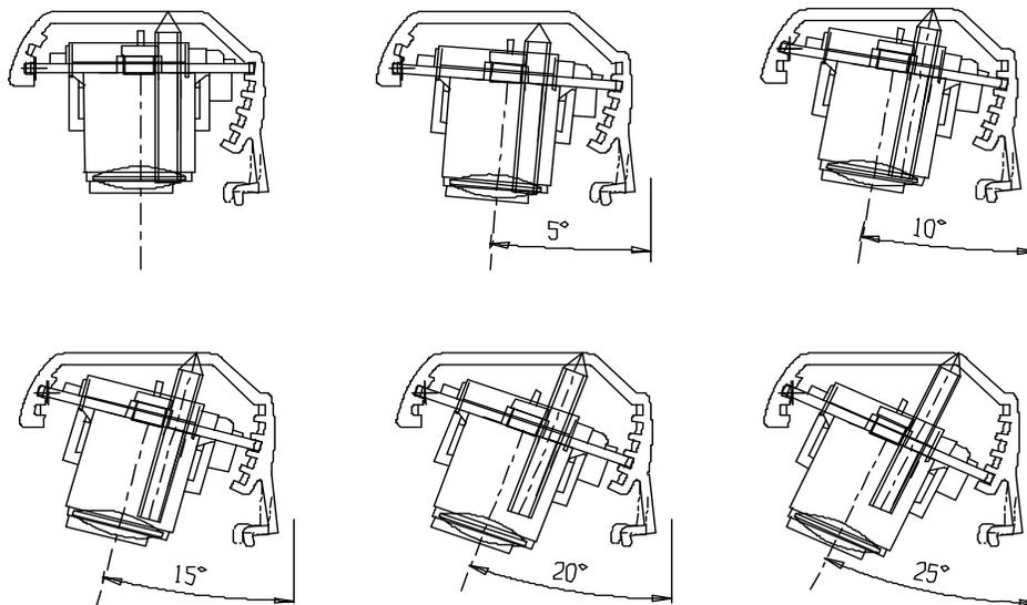
**POWER-ON POSITIONING, ANGLING AND ADJUSTING THE MODULES**
