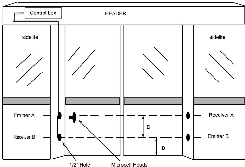
NOTE: Wire routing through breakaway sidelites
