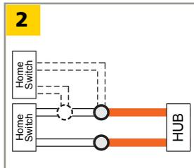
Wire nut white Home Switch wires to orange wires of System Harness plugged into hub<sup>2</sup>.
