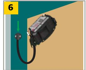
Install Door Loop: drill 1/2" passage hole in header and jamb, route Master Sensor Harness, install cap.
