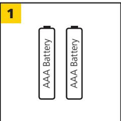
Replace 2 AAA batteries observing polarity.
