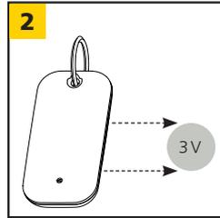
Replace 3-volt (CR2032) battery<sup>1</sup>, observing polarity, and reassemble.
