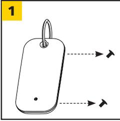
Remove back screws (2) and disassemble.
