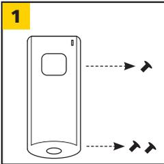
Remove back screws (3) and disassemble.
