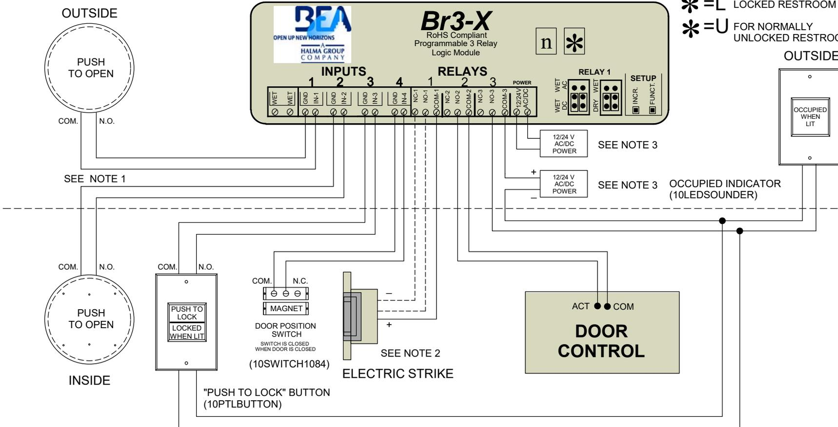
1) FOR INPUTS 1 & 2 ANY "DRY" CONTACT ACTIVATION DEVICE MAY BE USED.
