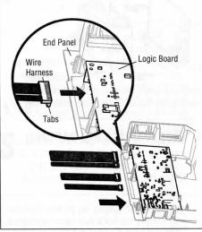
3.2 Insert the antenna wires through the holes in the end panel. Snap the receiver logic board into place on the end panel and fasten with screws.
