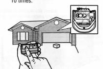
The garage door opener will not close from a remote control if the LED in either safety reversing sensor is off (alerting you to the fact that the sensor is misaligned or obstructed).
