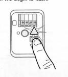
1.6 Press and release the UP Button. When the door travels to the programmed UP position, the DOWN Button will begin to flash.
