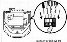
To insert or remove the wires from the terminal, push in the tab with a screwdriver tip.
