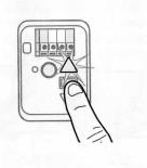
**1.2** Press and hold the UP Button until the door is in the desired UP position.
