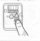
1.4 Press and hold the DOWN Button until the door is in the desired DOWN position.
