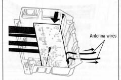
NOTE: Some models will require the short antenna wire to be placed in the traps of the end panel.
