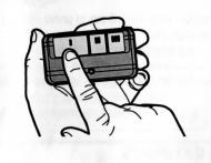
1.3 Release the button when the garage door opener light blinks. It has learned the code. If light bulbs are not installed, two clicks will be heard.
