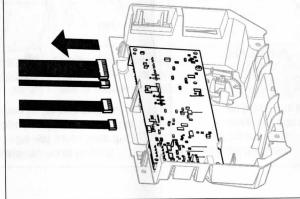
2.3 Remove the receiver logic board from the end panel by removing the 2 screws and releasing the 2 clips.
