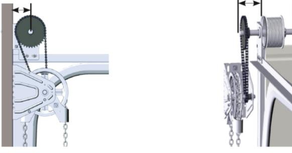
Chain hoist may be mounted on either side of the door
