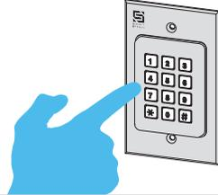
**7 Secure keypad unit to junction box using included screws.**
