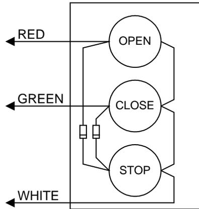
**This control station must be mounted a minimum of six (6) feet away from the gate and gate operator, or installed in such a way that the user cannot touch the gate or gate operator while using this control.**
