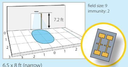
The size of the detection field varies according to the mounting height of the sensor.
