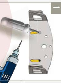
Remove the bracket from the sensor.
