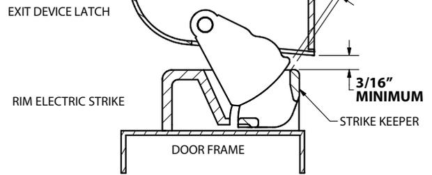
**NOTE:** Ensure a 1/16" [1.5mm] clearance between exit device latch and the electric strike keeper is maintained. Failing to do so will preload the strike and in turn will not allow the strike to release the door upon energizing.
