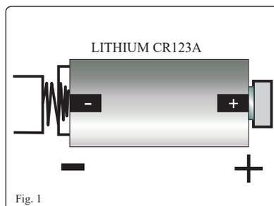
**NOTES:** The appliance uses a lithium battery type CR123A-S-3V. The removal and the disposal of the battery must have effected before the elimination of the appliance and according to the current Regulations. ATTENTION: - Danger of explosion if the battery is not replaced in the correct way! Replace only with an equal or equivalent type.
