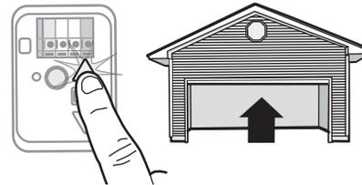
**1.7** Press and release the DOWN Button. The door will travel to the programmed DOWN position. Programming is complete.
