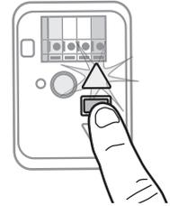
**1.4** Press and hold the DOWN Button until the door is in the desired DOWN position.
