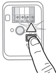
**1.6** Press and release the UP Button. When the door travels to the programmed UP position, the DOWN Button will begin to flash.
