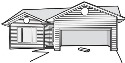
**2.2** Press the remote control push button to close the door. The door **MUST** reverse when it makes contact with the board.
