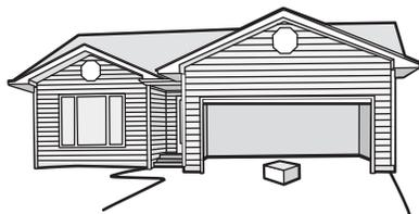
**3.2** Press the remote control push button to close the door. The door will not move more than an inch (2.5 cm), and the garage door opener lights will flash 10 times.
