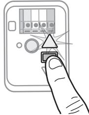
**1.2** Press and hold the UP Button until the door is in the desired UP position.
