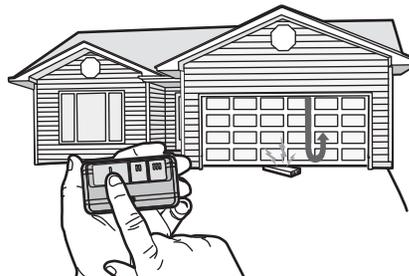
If the door stops and does not reverse on the obstruction, increase the down travel (refer to Adjustment Step 1).
